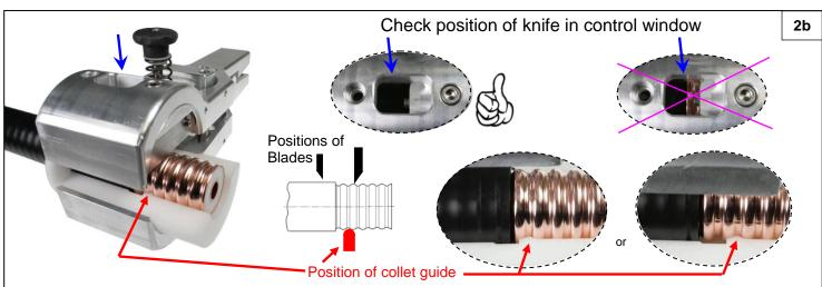
Keep the cable end downwards in order to prevent particles from entering during preparation.
