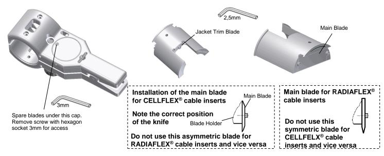
The blades are made of hardened steel. Therefore no commercially available cutting blades can be used as replacement. When the blades are worn-off replace with new blades.
